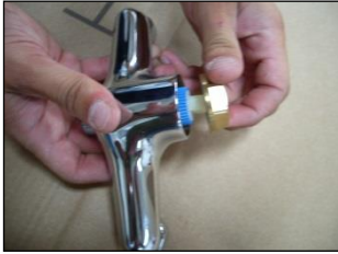
5 - unscrew the brass nut
